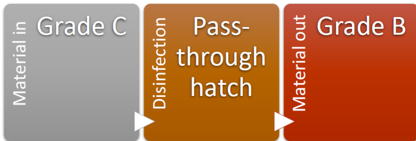
Figure 2: The pass-through cascade.
