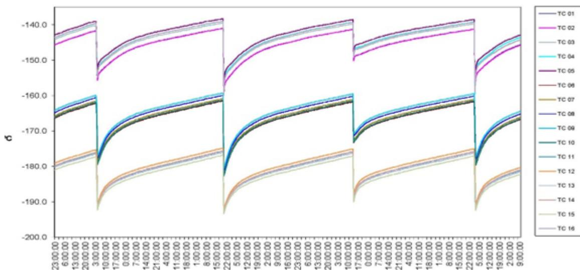
**Figure 4. This graph demonstrates planar temperature zones within the unit and shows stratification, trending colder at the bottom and warmer at the top of the unit. This graph also reveals at least three full cycles which complies with a best practice approach.**
