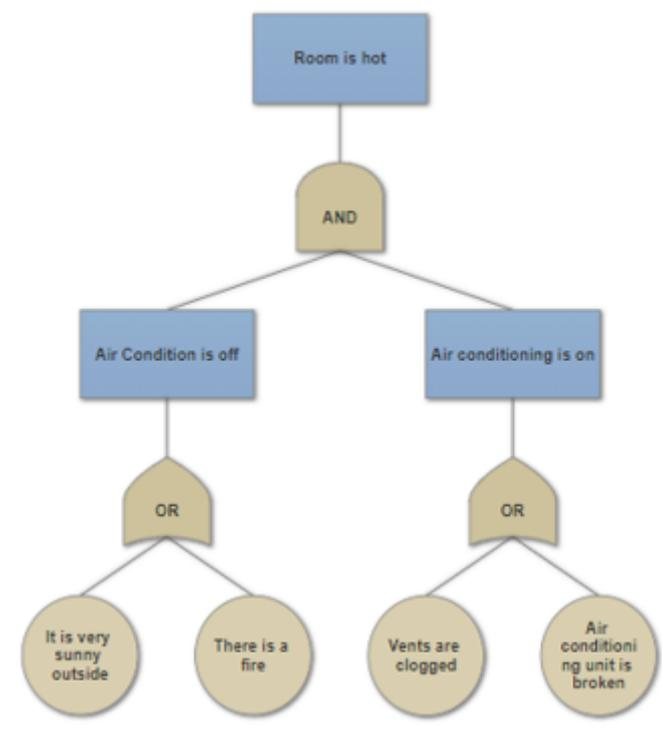
*Figure 2. Failure Tree Analysis Example*
