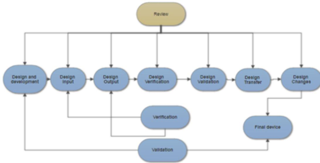
*Figure 1. Design Control Flow Chart*
